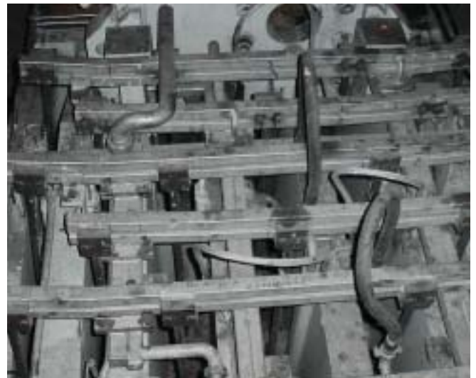
Vertical headers for MasterCooler SMART® air mist nozzles (Source: Hüttenwerke Krupp Mannesmann (HKM) Germany, 2-strand slab caster)
