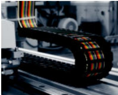
During long-term tests the System E3 with the spring band connector easily passes 15 million cycles at a bending radius of 44 mm and an acceleration of 4 g
