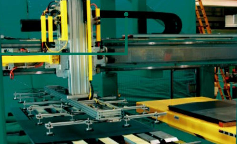
A linear drive provides for highly dynamic feed of PCBs. This system is twice as fast as handling units with a toothed-belt drive; designed to withstand high dynamic loads, the E6 e-chains® ensure a supply of power, coolant and control data with ultra-low noise and vibration
