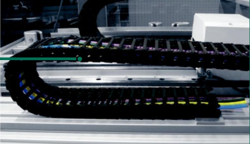
Long-term tests in our acoustics laboratory at a speed of 1.8 m/s and an acceleration of 3 m/s<sup>2</sup> showed reductions of 19-20 dB(A) compared to conventional e-chains®.
