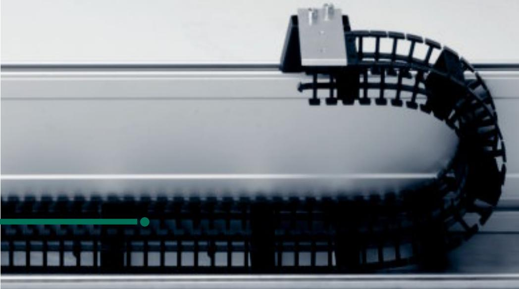
Extremely low noise - System T3 tests in the igus® lab at 1 m measuring distance showed a value of = 33 dB(A) at 26.5 dB(A) basic sound level for Series T3.29.050.038
