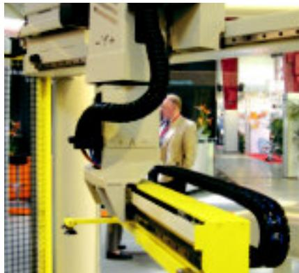
igus® System E6 and triflex® R TRE in a Y/Z-gantry
