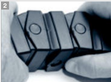
Snap in pin "push-button-principle"
