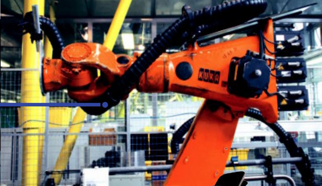
**triflex® RS - universal module for safe realisation of complex robotic movements**
