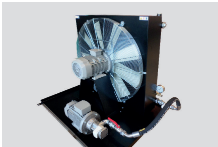
Lube oil cooling system
